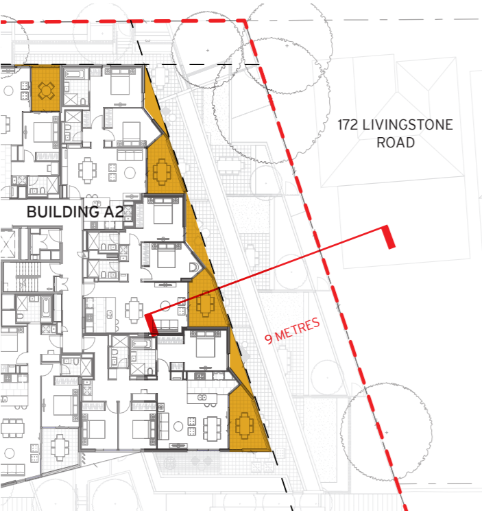
BUILDING A NORTH BOUNDARY PLAN AT TYPICAL LEVEL (L04) ARTICULATION ZONE SHOWING EFFECTIVE SETBACK OF GLAZING & DEEP BALCONIES, WHICH PROVIDES GREATER AMENITY FOR BOTH PROPOSED RESIDENTS AND EXISTING NEIGHBOURS
