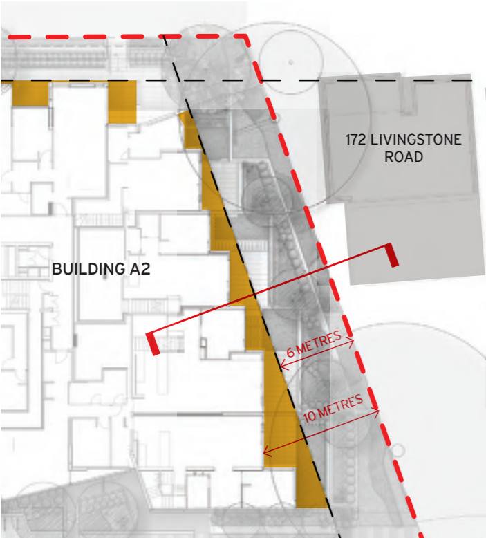
BUILDING A NORTH BOUNDARY PLAN AT GROUND LEVEL ARTICULATION ZONE SHOWING EFFECTIVE SETBACK OF GLAZING
